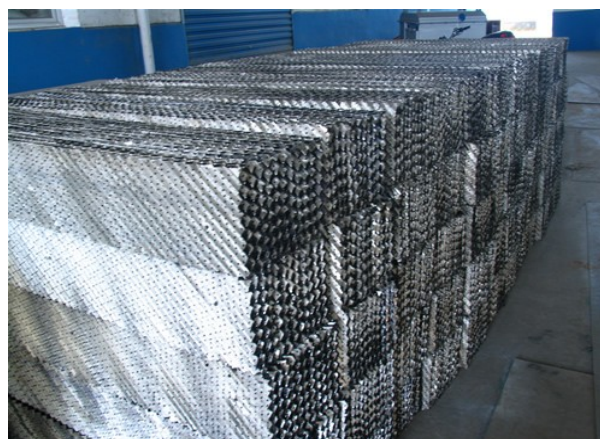
Illustration 3: Metal Structured Packing(KPK-MSP)
